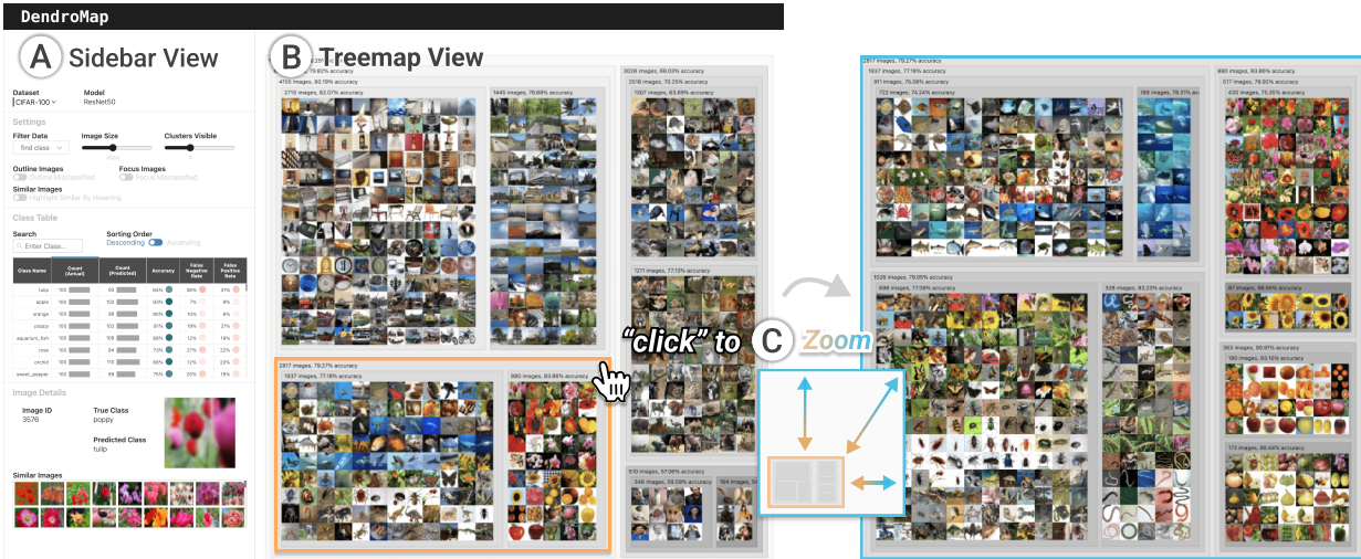
Fig. 1. With DendroMap, users can explore large-scale image datasets by overviewing the overall distributions and zooming down into hierarchies of image groups at multiple levels of abstraction. In this example, we visualize images of the CIFAR-100 dataset by hierarchically clustering the image representations obtained from a ResNet50 image classification model. (B) Treemap View displays these clusters of images organized as a hierarchical structure by adapting Treemaps. By clicking on a cluster, a user can interactively (C) Zoom into that image group, revealing subgroups that replace and fill the available space with animation. The user clicked on a cluster for organism images, which creates distinct subgroups of fish, insects, fruits, and flowers. With (A) Sidebar View , the user can dynamically adjust the number of clusters to be displayed and inspect the class-level statistics.
